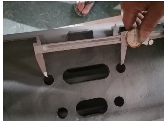
Longitudinal / lateral bolt spacing reference
